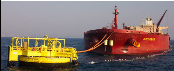
Single Point Mooring (SPM) – weather-vaning systems
