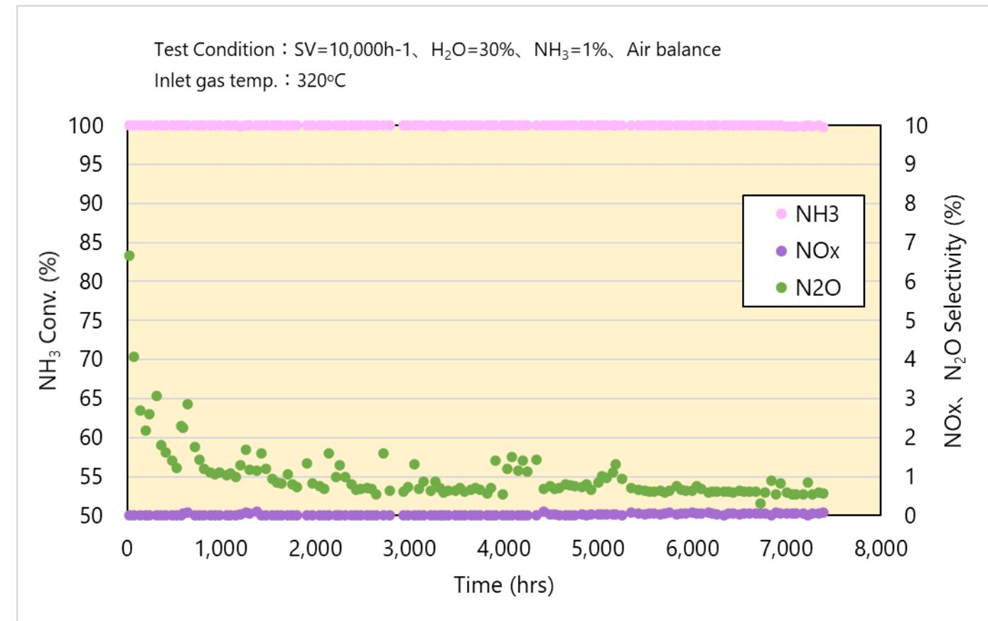
**NH<sub>3</sub> destruction catalyst can treat NH<sub>3</sub> with almost no NOx formation and minimized N<sub>2</sub>O formation. Long-term stability of NH<sub>3</sub> decomposition performance under high moisture level was confirmed.**
