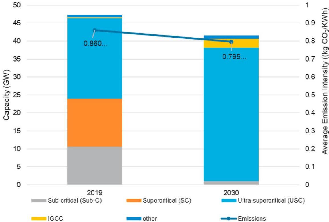
Capacity mix of thermal coal power generation technology and emissions intensity for 2019 and ANRE 2030 proposal.
