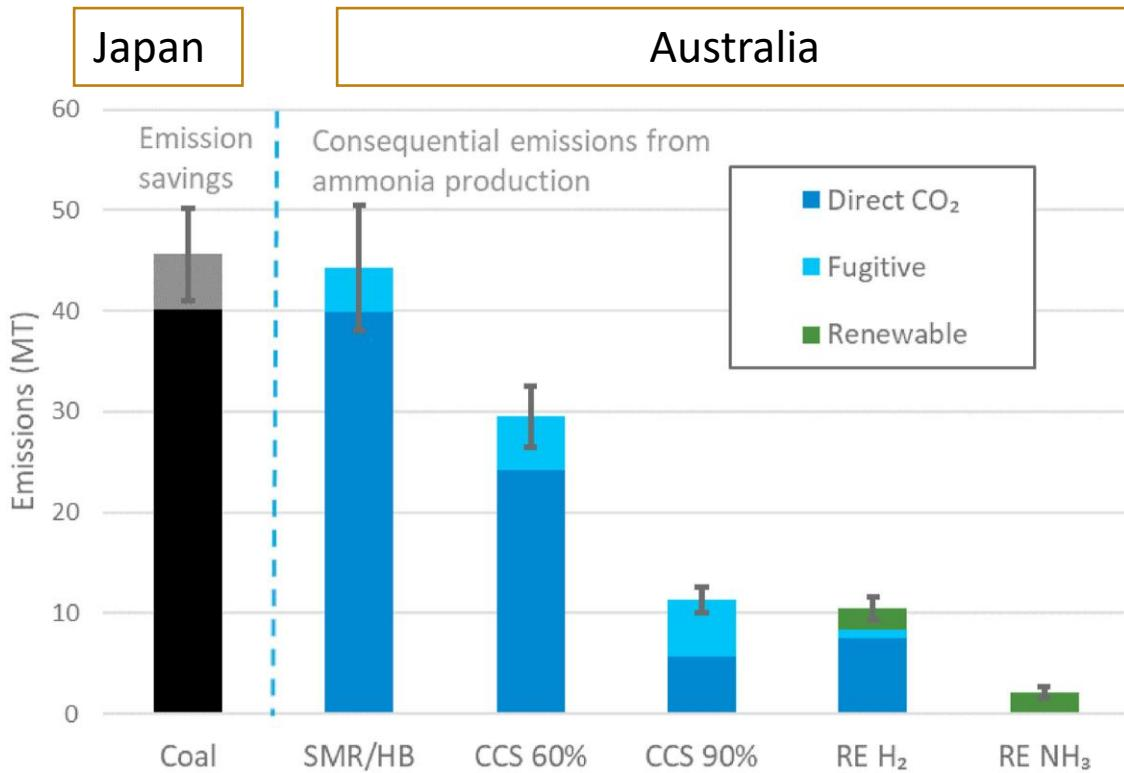
Annual emissions savings due to 20% ammonia/coal co-combustion in Japan's 2030 coal fleet, consequential emissions from ammonia production in Australia.
