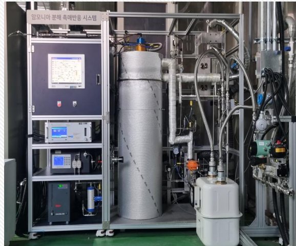
\text{NH}_3 decomposition reactor ( \text{H}_2 20 \text{Nm}^3/\text{h} )
