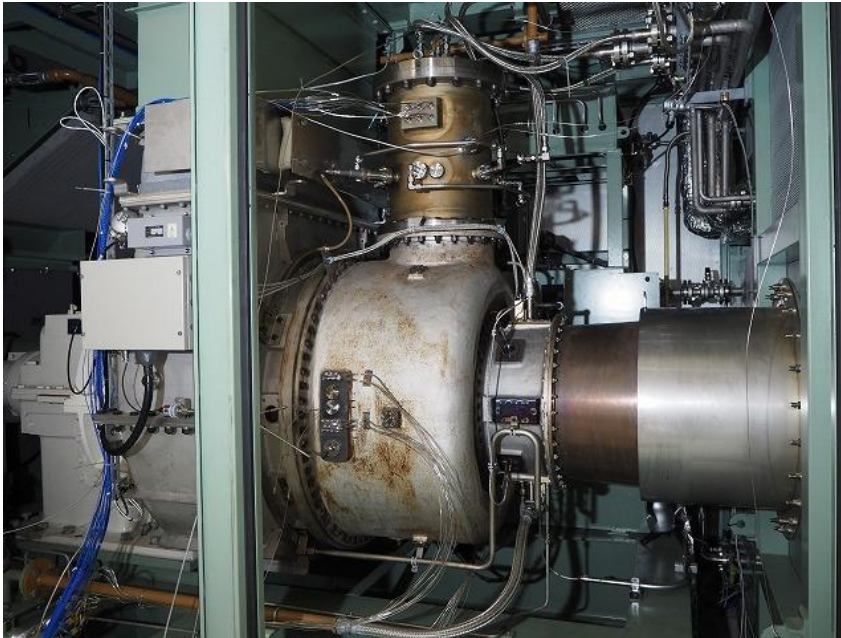
2MW class ammonia fueled gas turbine (IM270)
