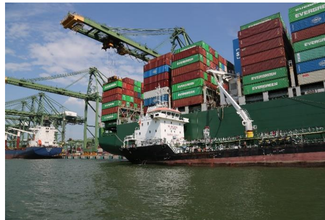
Ship to ship bunkering with simultaneous cargo handling (SIMOPS)
