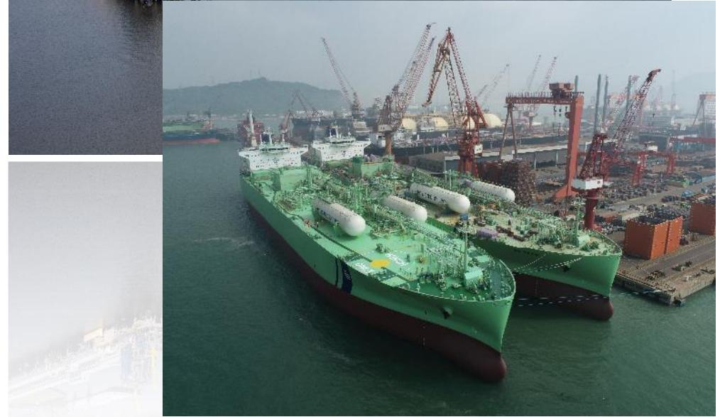
\*Pictures courtesy of BW Gas. 15 VLGCs will be retrofitted to LPG propulsion with MAN B&W engines.
