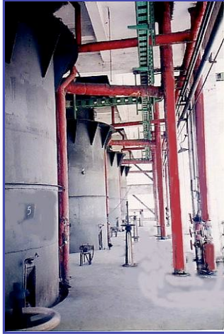
5 operating gasifiers installed in 1992
