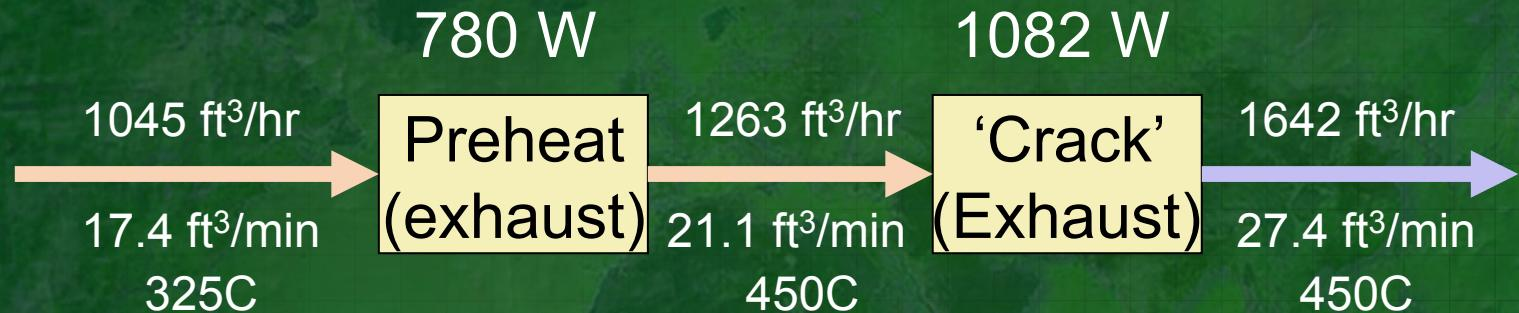
$$.265 \text{ whr/lbC} \times 125 \text{ C} \times 23.54 \text{ lb/hr} = 780 \text{ W}$$
