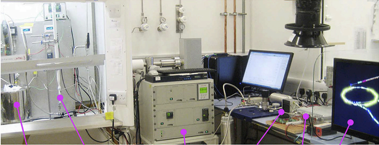
\text{NH}_3 cracker (reactor) purification column mass spectrometer PEM fuel cell fuel cell controller TV (powered by fuel cell)
