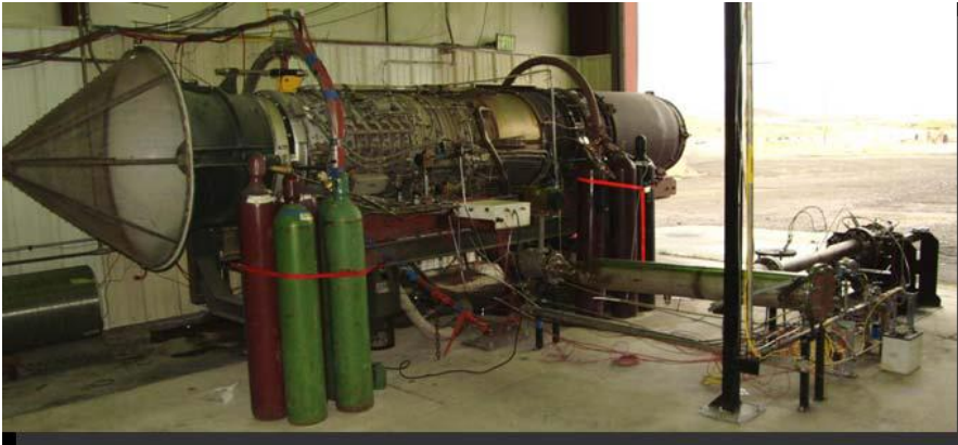
\text{NH}_3 -air combustion gas turbine (Evans, 2013)
