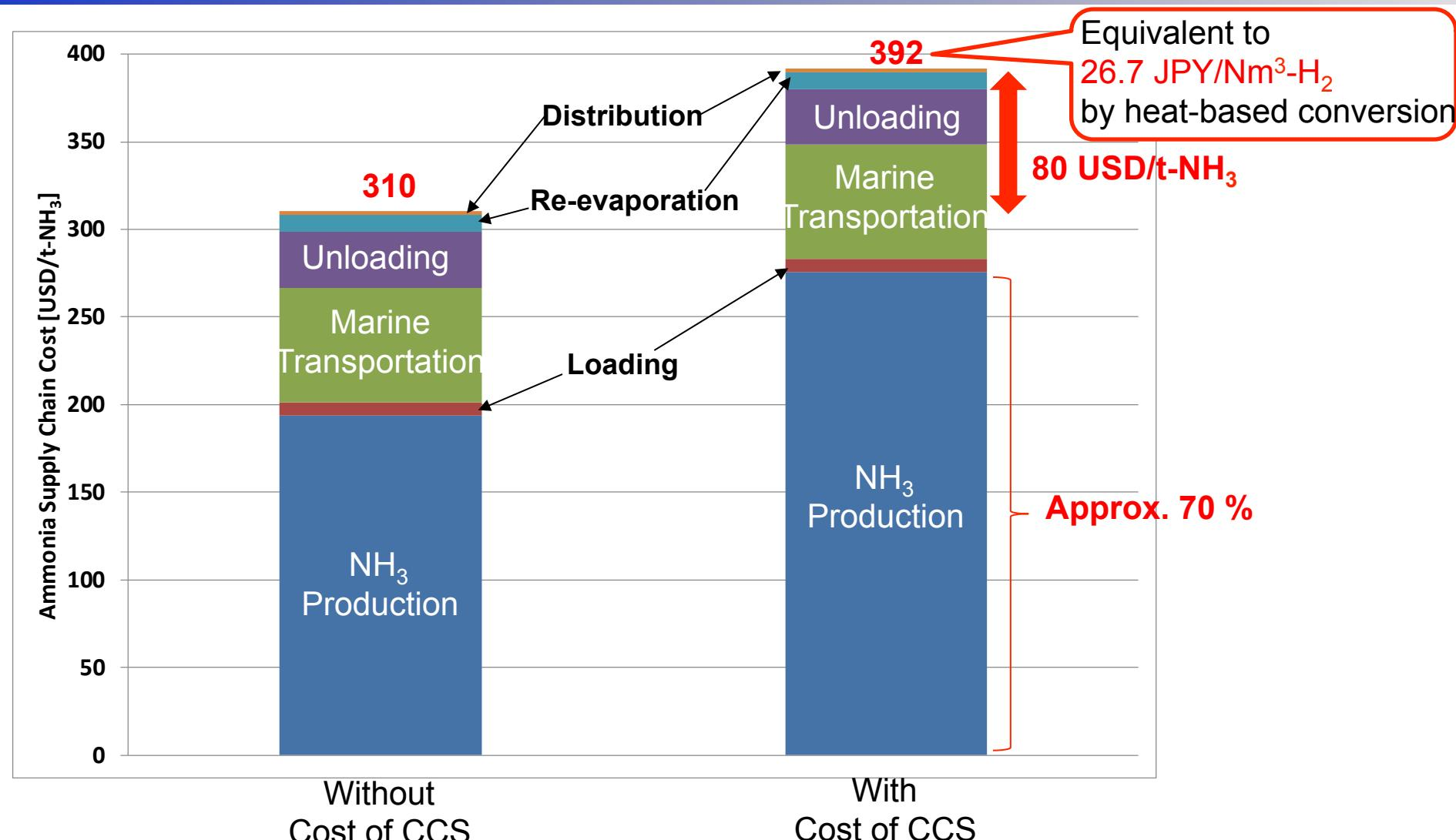
Estimated NH<sub>3</sub> supply chain cost is lower than the target of H<sub>2</sub> cost (30 JPY/Nm<sup>3</sup>-H<sub>2</sub> in 2030) from "Basic Hydrogen Strategy", Japan
