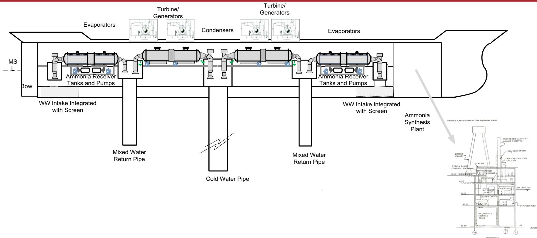
**75 MWe with NH<sub>3</sub> capacity of 200 MTD with provision of disconnecting CWP and move the platform in the event of hurricane**
