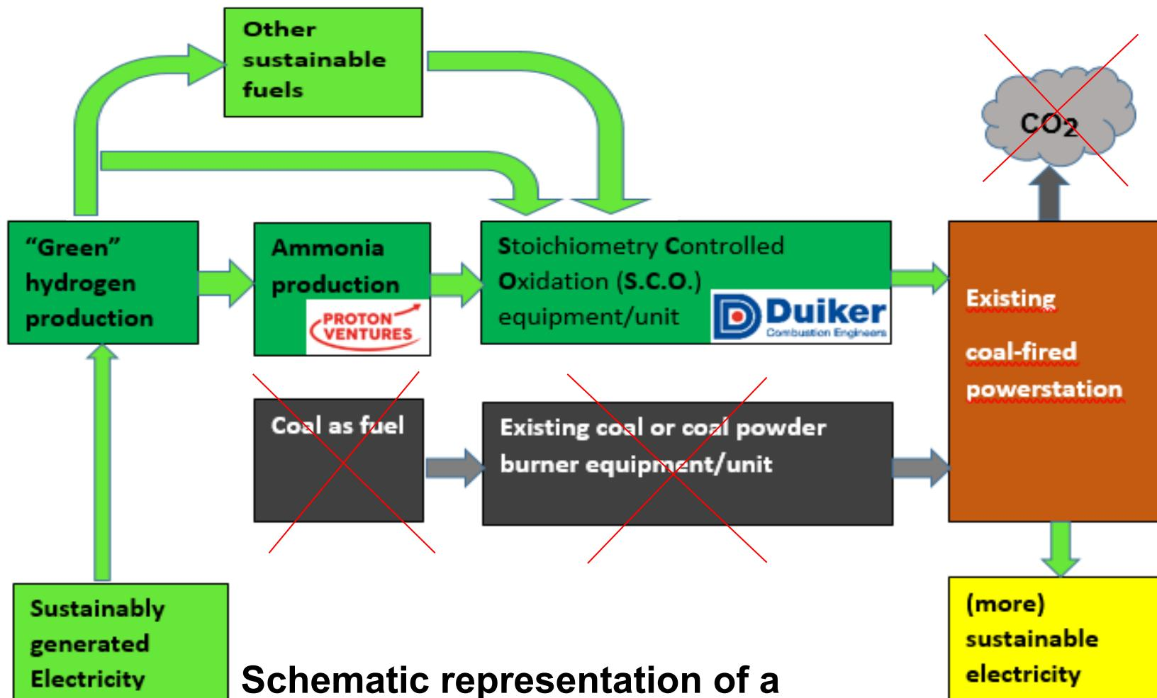
**Schematic representation of a sustainable multi-fuel coal-fired power station**
