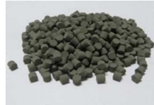
Ru/CeO 2 catalyst produced on a semi-industrial scale
